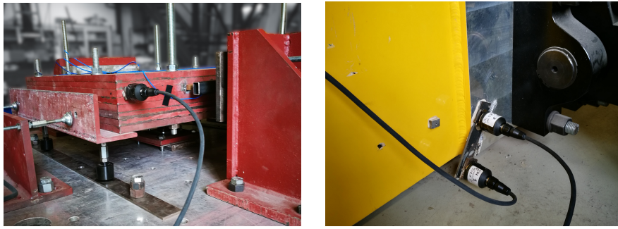
Figure 2.11. Accelerometers: a mass; b table.
