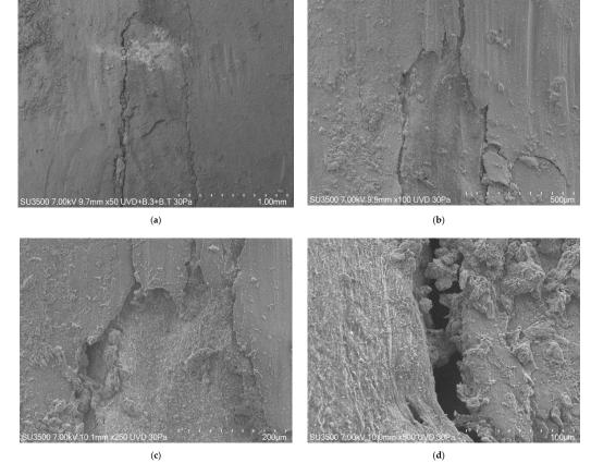
Figure 2. Gap observation of wet samples at four different magnifications. (a) 1 mm; (b) 500  $\mu$ m; (c) 300  $\mu$ m; (d) 100  $\mu$ m.
