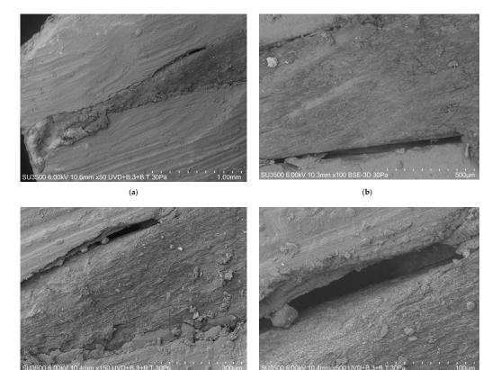
Figure 1. Gap observation of humid samples at four different magnifications. (a) 1 mm; (b) 500 μm; (c) 300 μm; (d) 100 μm.
