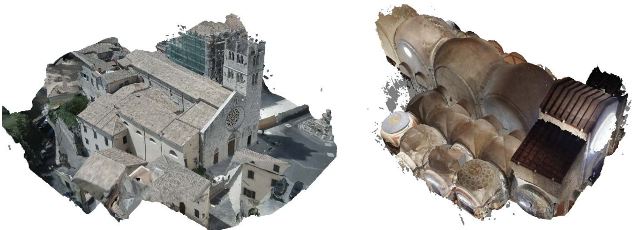
160 Figure 4 – High-density point cloud with applied texture of the: a) exterior; and b) interior of the church of Santa Maria 161 Maggiore.
