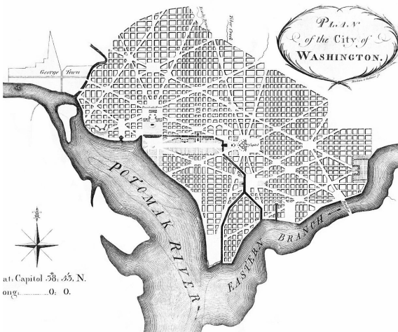
Fig. 17 Andrew Ellicott's plan for Washington depicting the Washington City Canal that connected the Potomac River, Tiber Brook and C&O Canal to the East Branch (Anacostia River) Source: Library of Congress, Andrew Ellicott's initial Plan of the City.
