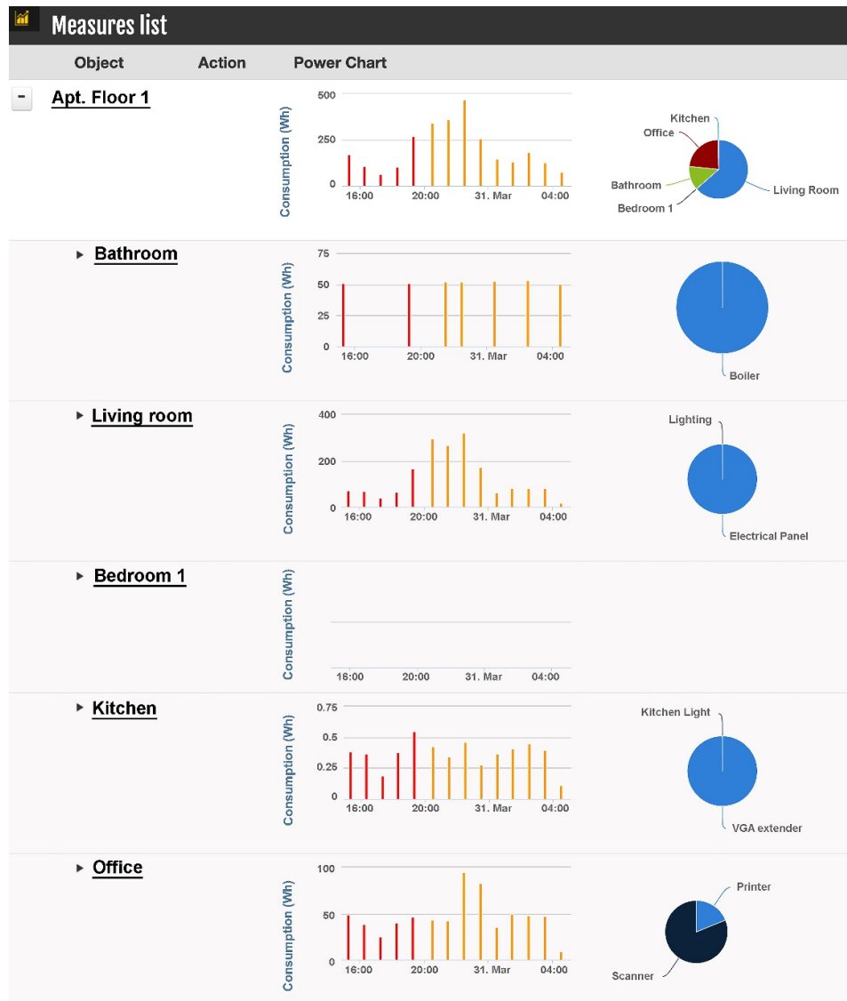
Figure 18. Submetering in a typical apartment.
