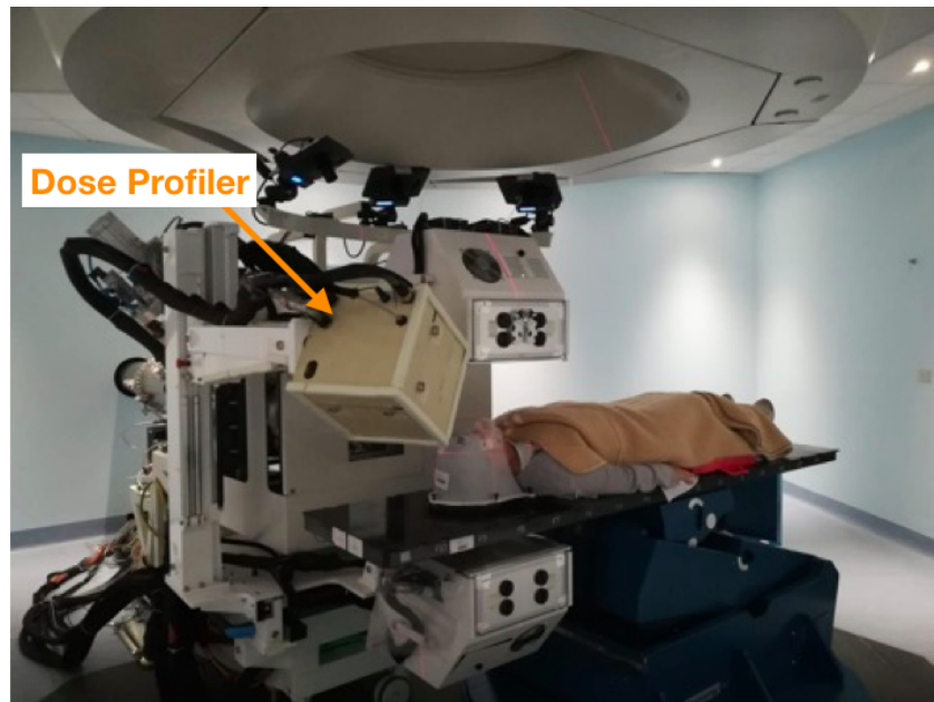
Figure 2.11. Photo of the first clinical trial of the Dose Profiler during a carbon ion treatment of a head tumor at CNAO [63].
