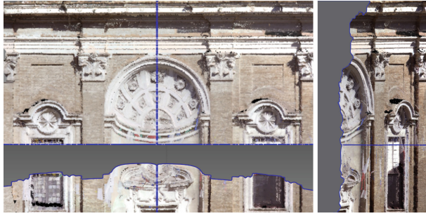
Fig. 8. Horizontal and vertical section on the perspective niche (model by M. Carpiceci)
