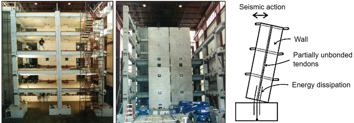
Figure 4.2. Left and centre: Five-Storey PRESSS Building tested at University of California, San Diego (Priestley et al. 1999); Right: concept of low-damage system (fib 2003).
