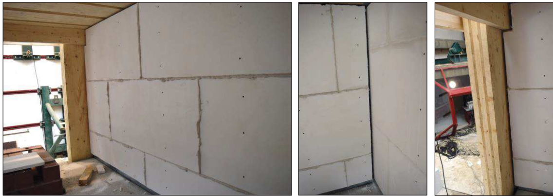
Figure D.7. Partition in the frame direction: complete assembly of the wall (left); gap between the two orthogonal walls (centre); gap between the partition and the timber wall (right).
