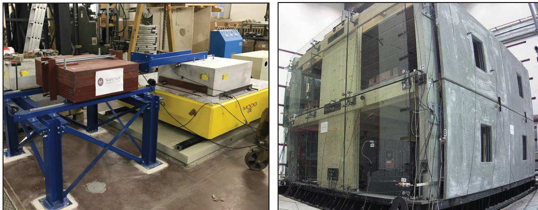
Figure 10.2. Left: Experimental campaign carried out at the Structural Laboratory of the University of Rome on post-installed anchors; Right: Experimental campaign carried out at the Laboratório Nacional de Engenharia Civil (LNEC) in Lisbon - Phase 3 of experimental testing.
