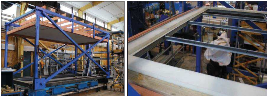
Figure 4.10. Test specimen (left) and detail of isolation foam placed in the lateral gap (right) (Pourali et al. 2017).
