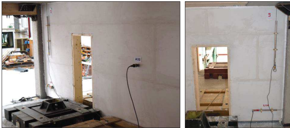
Figure 7.9. Instrumentation plan for the partition in the wall direction: schematic drawing (top) and photos (bottom).
