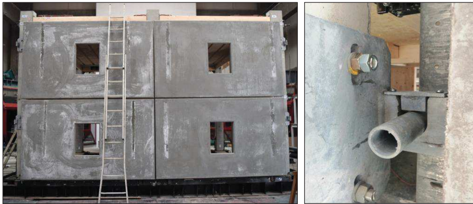
Figure 6.38. Final configuration of the GFRC façade (left) and of the upper sliding anchorage (right).
