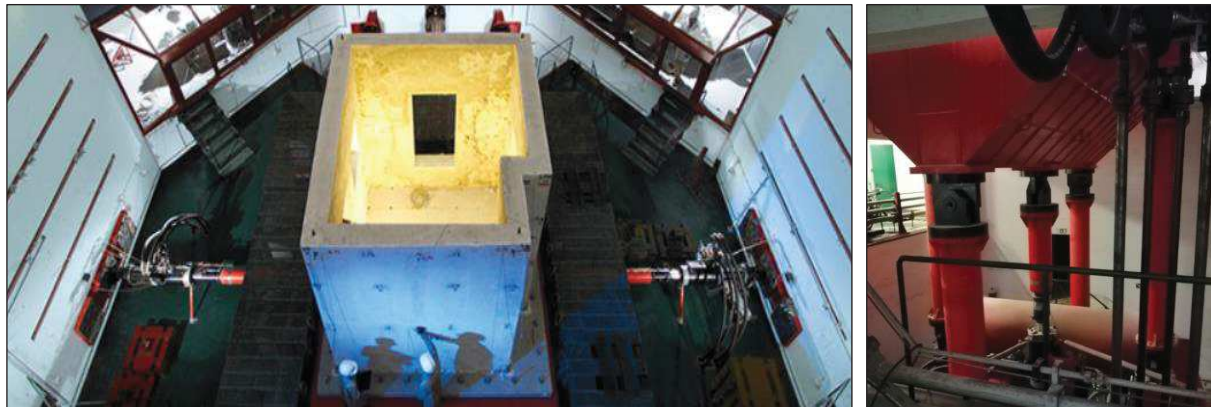
Figure 7.1. Shake-table of the Laboratório Nacional de Engenharia Civil (LNEC): top view (left) and vertical hydraulic actuators (right).
