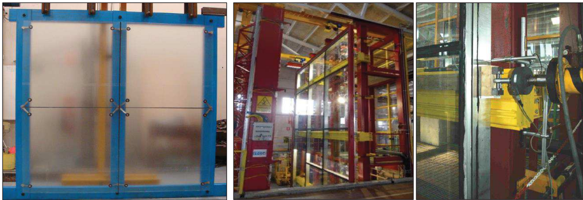
Figure 3.13. Left: experimental tests on spider glazing configurations (Sivanerupan et al. 2010); Right: Test setup of a full-scale stick curtain wall and lateral load application by a hydraulic jack (Caterino et al. 2017).
