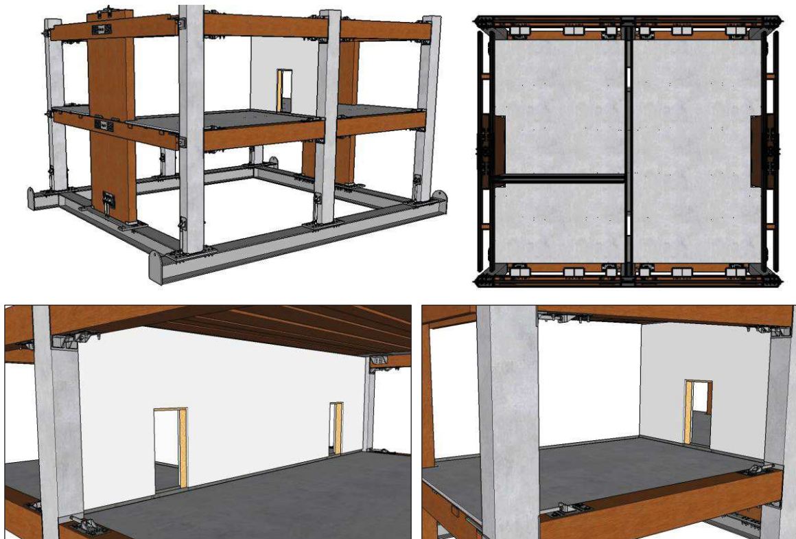
Figure 6.11. Renders of Option 1 configuration: global view (top - left), distribution in plan of the partitions (top - right), view of the wall with openings (bottom - left), view of the wall without openings (bottom - right).
