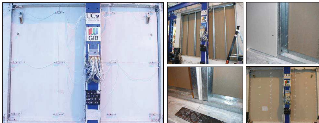
Figure 4.9. Left: experimental test on the low-damage drywall system (Tasligedik et al. 2014); Right: details of the wall construction (top-left: sub-frame system; bottom left: friction fitted interior fire-rated stud; top-right: installation of the gypsum lining to the steel studs; bottom-right: finished drywall partition) as described in Tasligedik (2014).
