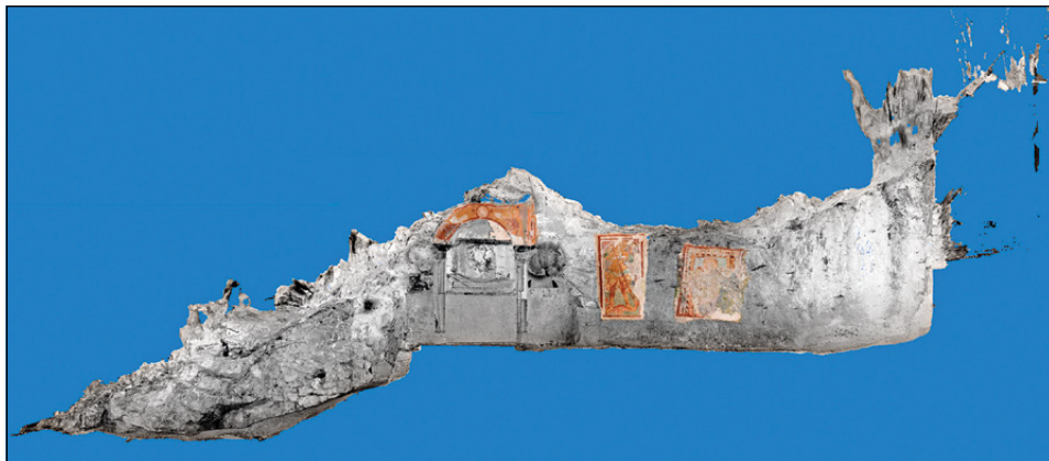
Fig. 3 – Different scans were performed in order to survey the entire cave and to have a complete numerical model of the whole pictorial cycle.
