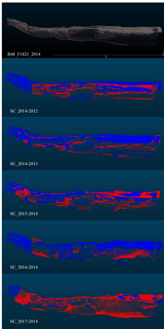
Fig. 7. Building 48, Point cloud of Feature 1821 in 2014 (above) and the variation of Significant Change areas as outlined in CloudCompare, from 2012 to 2017 (below). Red points show change while blue points indicate no significant change.
