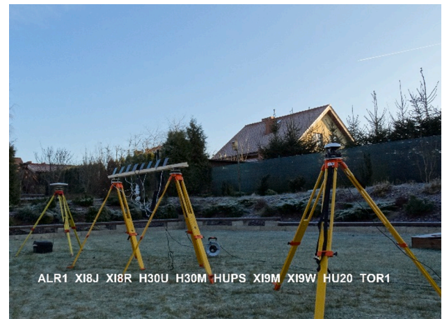
Fig. 1. Smartphones and geodetic receivers during data collection. Location of the smartphones and receivers correspond to the order of RINEX IDs given in the bottom of the figure (c.f. Table 1). During data collection SIM cards were not inserted in the smartphones.
