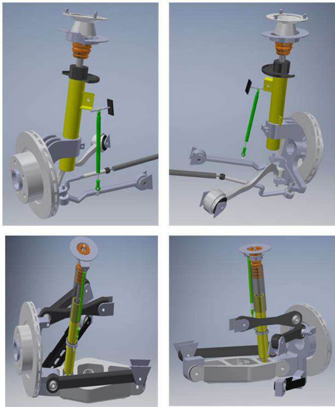
Figure 10. CAD of the original BMW front kinematic suspension at the front (top) and the rear (bottom).
