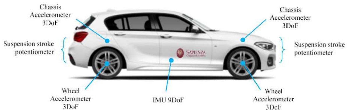
Figure 4. Sensors positions on BMW series 1.
