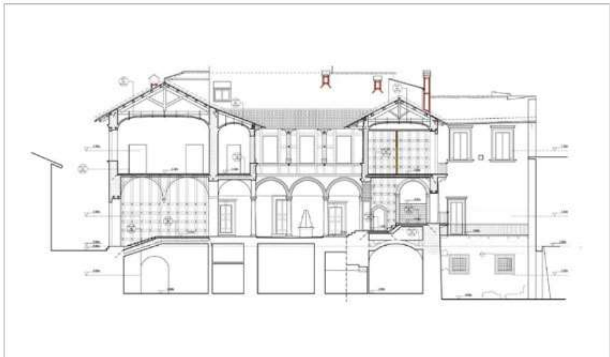
Fig. 14. The consolidation project: the section along the courtyard shows the reinforces on the more damaged walls (drawing by F. De Cesaris, 2012)
