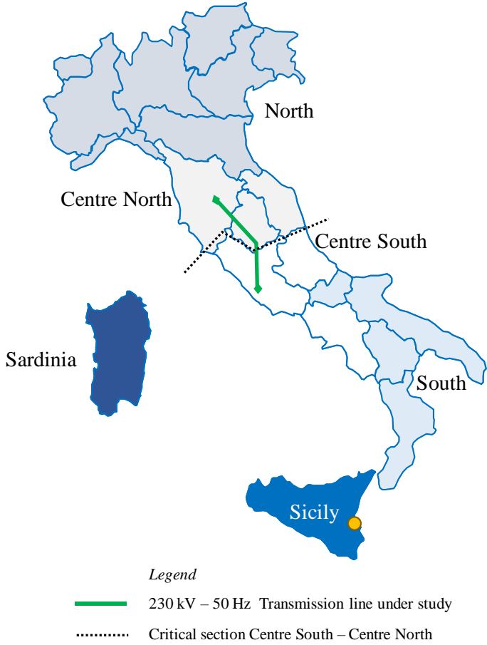
Fig. 1.1. Market zones of the Italian power system (year 2018) with the f 230 kV transmission line under study.
