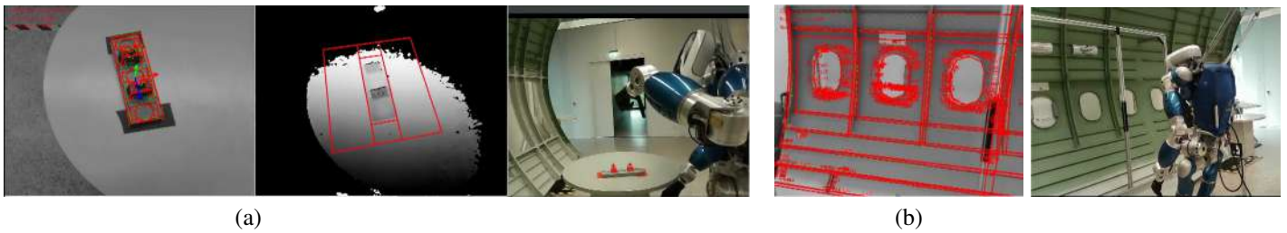
Fig. 4: Visual tracking results obtained with TORO: (a) bracket tracking using edges and depth (left: image with edges extracted and model projected from the estimated pose, middle: depth map with model used projected from the same pose, right: robot configuration), (b) fuselage tracking using edges and key-points with TORO (left: image with edges and key-points used and model projected from the estimated pose, right: robot configuration).
