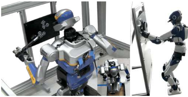
Fig. 14: Narrow access in multi-contact and fast dynamic torqueing handling four contacts with HRP-2Kai. (left). Circuit breaker checking combining multi-sensory task-space control with HRP-4, achieved without visual markers (right).
