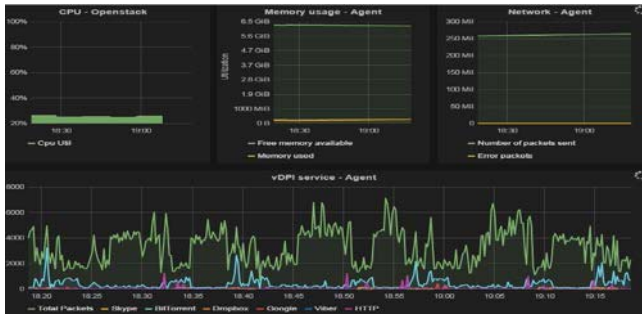
Fig. 12. GUI screenshot aggregating metrics from various sources to monitor a vTC VNF.
