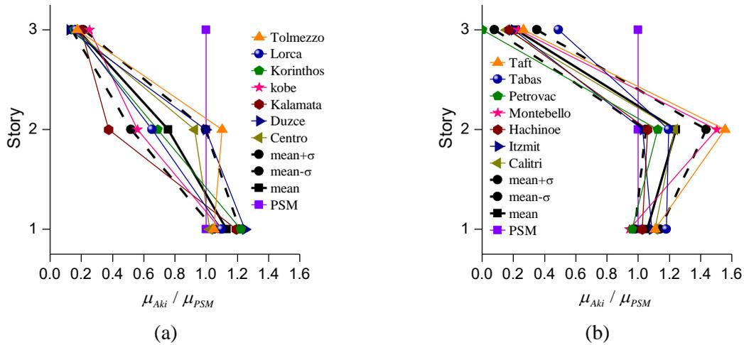
Figure 7.  $\mu_{Aki,i}$  normalized by  $\mu_{PSM,i}$  for the 3-story building using: (a) near field records; (b) far field records
