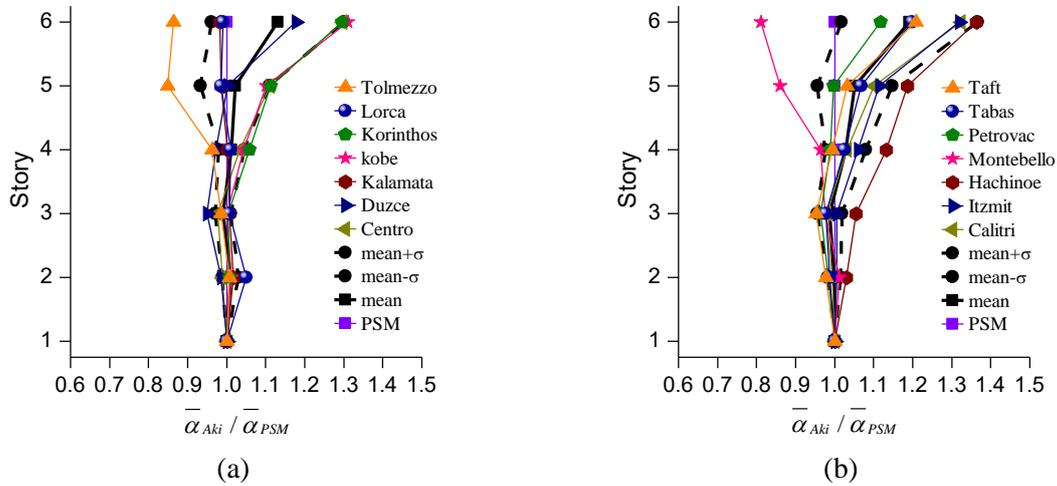
Figure 4.  $\bar{\alpha}_{Aki,i}$  normalized by  $\bar{\alpha}_{PSM,i}$  for the 6-story building using: (a) near field records; (b) far field records
