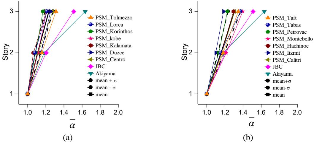
Figure 1.  $\bar{\alpha}_i$  obtained for the 3-story building using: (a) near field records; (b) far field records
