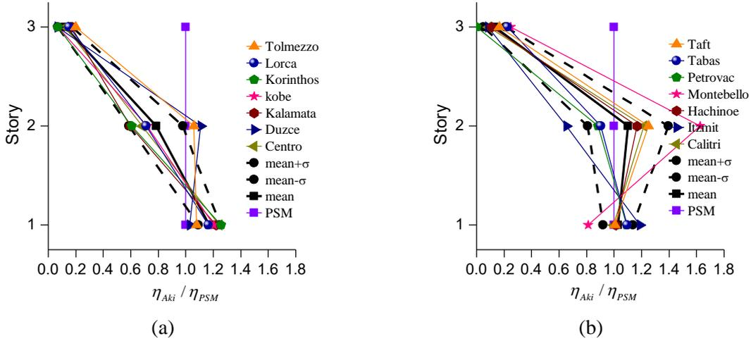
Figure 5.  $\eta_{Aki,i}$  normalized by  $\eta_{PSM,i}$  for the 3-story building using: (a) near field records; (b) far field records
