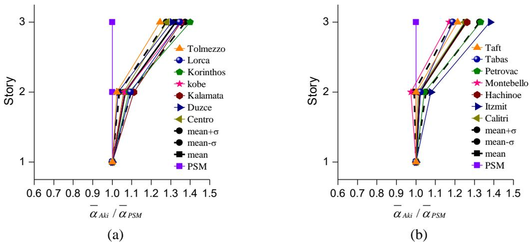
Figure 2.  $\bar{\alpha}_{Aki,i}$  normalized by  $\bar{\alpha}_{PSM,i}$  for the 3-story building using: (a) near field records; (b) far field records
