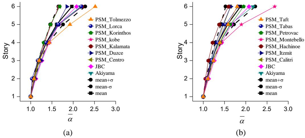
Figure 3.  $\bar{\alpha}_i$  obtained for the 6-story building using: (a) near field records; (b) far field records
