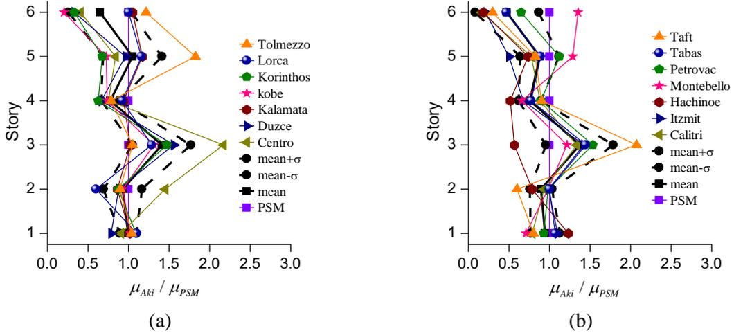
Figure 8.  $\mu_{Aki,i}$  normalized by  $\mu_{PSM,i}$  for the 6-story building using: (a) near field records; (b) far field records
