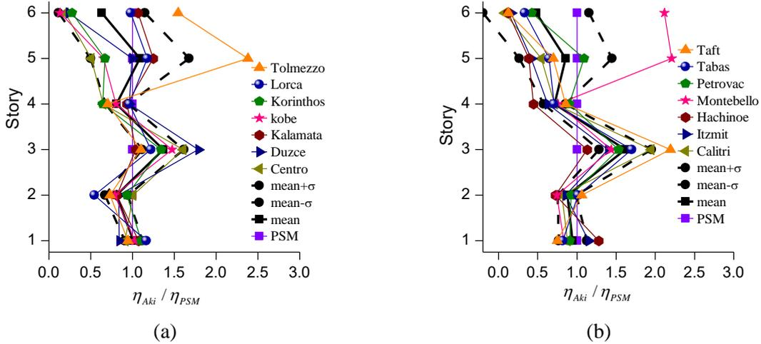
Figure 6.  $\eta_{Aki,i}$  normalized by  $\eta_{PSM,i}$  for the 6-story building using: (a) near field records; (b) far field records
