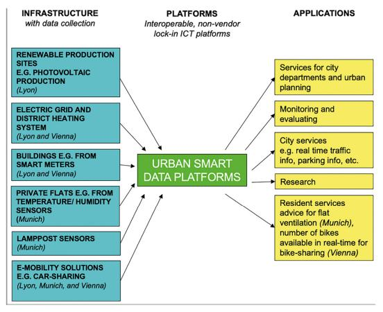
**Figure 4.** Data flow within the established data management platforms for the three LHCs. From left to right: Infrastructure components as inputs (turquoise), smart data platform repository and analysis (green), and applications as outputs (yellow).
