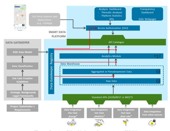
Figure 2. Overview of Munich's data gatekeeper registry to SDP [20].
