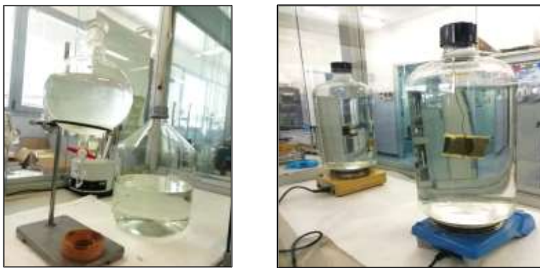
Figure 20 Left: Reference method: LLE; Right: ACF method
