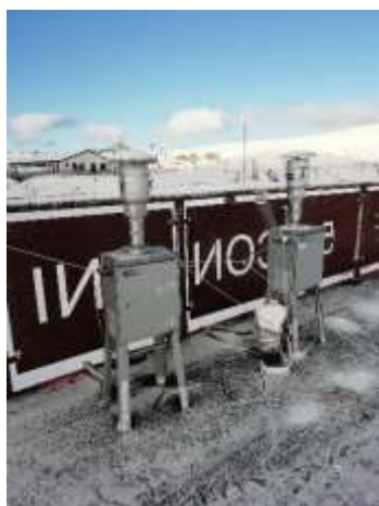
Figure 31 Parallel High Volume PM 10 Sampler, HV A and HV B
