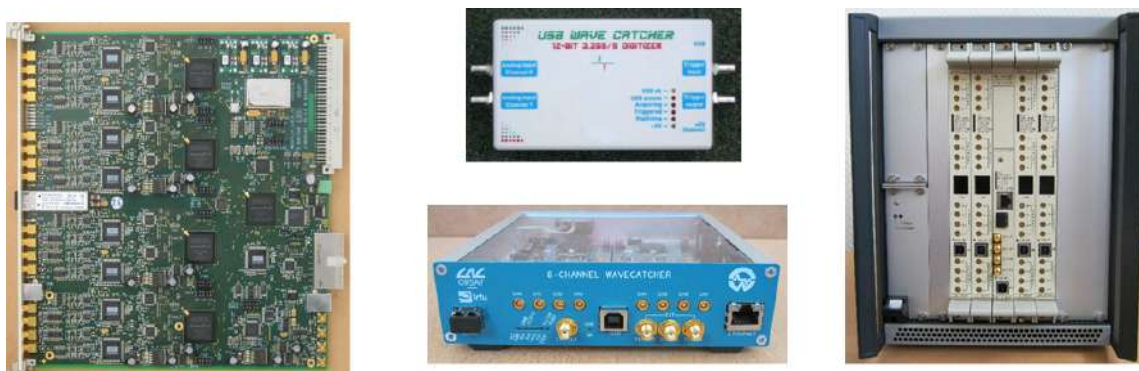
Figure 11. Left: 16-channel WaveCatcher board — Middle: 2-channel USB and 8-channel WaveCatcher module — Right: crate composed of 6U custom-board which can be integrated in a small crate controlled by a dedicated board in order to reach up to 64 channels.
