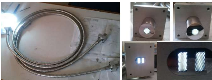
Figure 26. The 4 m bundles composed of 100 fibers each. The ends of the bundles match the shapes of the Quartz bars (rectangle) and of the PMT window (round).
