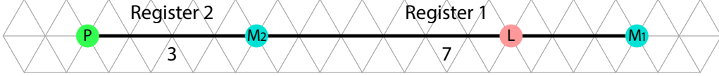
Fig. 2: A RAM simulator with the first register holding the value 7 and the second register holding the value 3.
