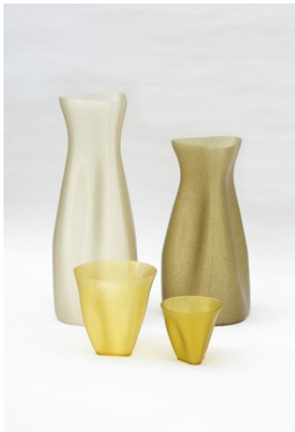
Fig.1 “Algae Lab” by Atelier Luma. 3d Printed pots realized with filament derived from algae of different geographic areas. [Antonelli, P. & Tannir, A. (2019). Broken Nature. XXII Triennale di Milano. Electa: Milano].
