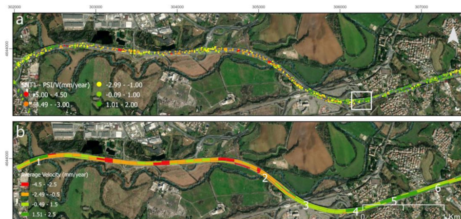
Figure 10. (a) Displacement map PSI Sentinel-1 A24 highway, (b) Map classification sections average velocity (mm/year) and bridge 1-6, as background ESRI source 2020.
