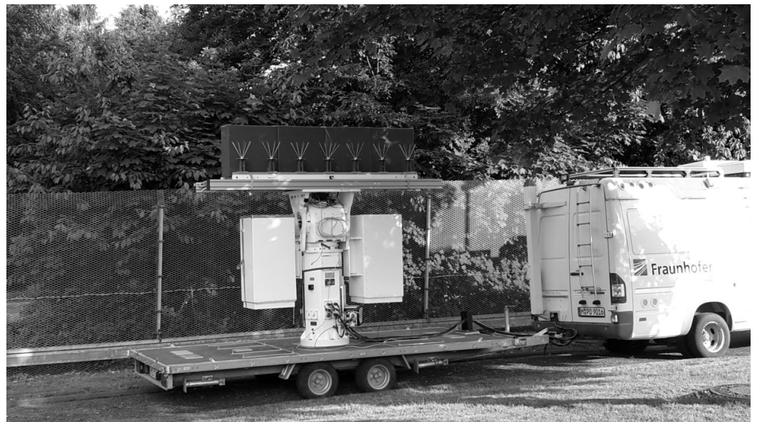
Figure 7. Picture of the bus with the trailer as the carrier platform. The uniform linear array is mounted on top of the white pedestal and steered along-track in the right-looking condition. The Radiation Absorbing Material (RAM) shielding the antennas to one side can be seen on top of the pedestal behind the antenna array.
