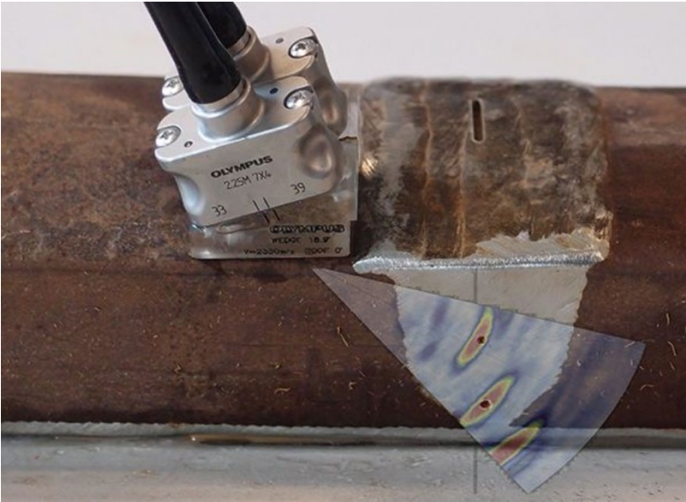
Figure 2: Ultrasonic testing to find welding cracks
