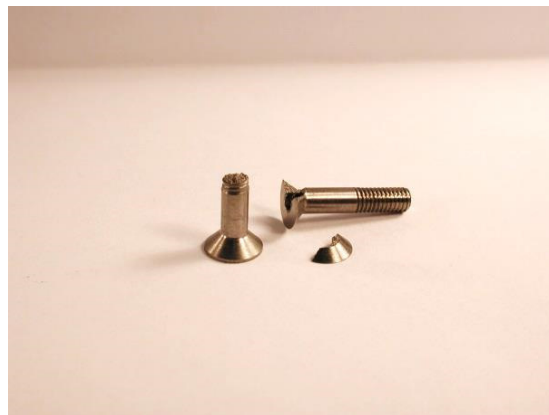
Fig. 3. Macrograph showing the broken screws
