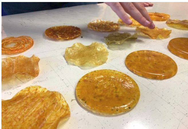
Fig. 2 Examples of DIY bioplastic produced using food scraps from traditional local delicacies of Lazio Region.
