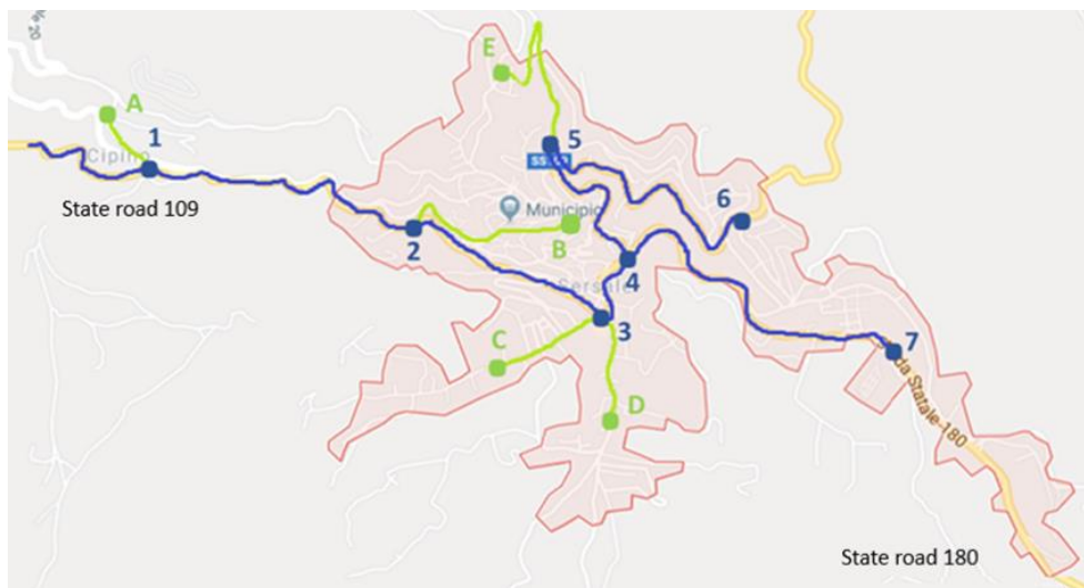
Figure 18. Path of the main pipelines (blue) and the secondary branches (green) of the DHN.
