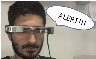
Fig. 5. Example of auditory prompts provided for people with visual impairment. The HMD will read out the message “Alert”.
