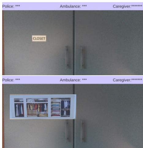
Fig. 4. Top image: the marker is applied on the closet door. Bottom image: when the user looks at the marker (the label), an image appears on the display representing the contents of the closet, without having to open it.
