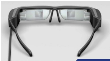
Fig. 6. Si-OLED (Silicon - Organic Light-Emitting Diode) display is able to show the visual prompts, useful for people affected by hearing impairment.
