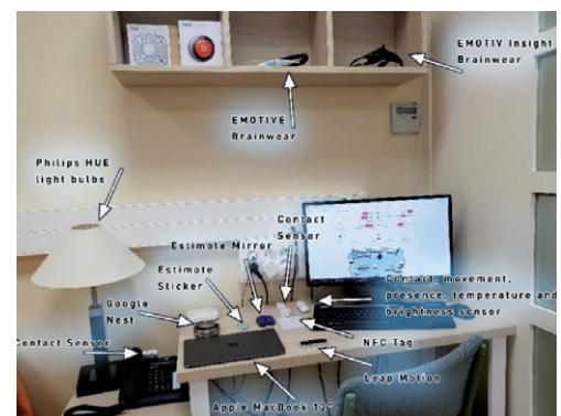
Fig. 14-19 | UJAml.prototype model: a review of sensors and actuators integrated with the home environment (source: www.remind-research.com).
