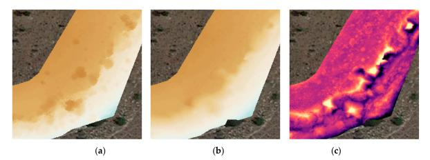
**Figure 5.** Details of (**a**) the DEM, (**b**) the DTM, and (**c**) the difference between the original and smoothed DTM, which shows that the point cloud contains a relatively narrow depression under a small tree.
