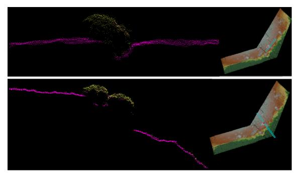
**Figure 6.** Sections of the classified point cloud corresponding to relevant site #1. **Above**: section approximately in the direction of the edge of the plateau; **below**: section approximately across the edge. The cyan boxes in the top views displayed on the right of the panels indicate the position and extension of the sections. Red points indicate the approximate location of the point of interest (coordinates were taken manually for the purpose of locating the points on the ground).
