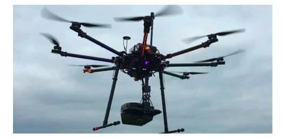
Figure 2. The Yellowscan Mapper LiDAR flying under the octocopter.
