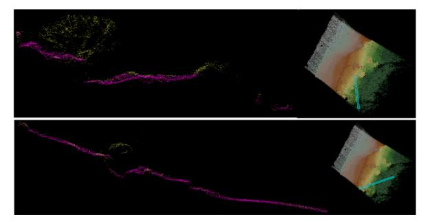
**Figure 7.** Sections of the classified point cloud corresponding to relevant site #2. Sections were taken along two orthogonal directions not directly oriented with the edge of the plateau (**above**: section taken approximately in the North-South direction; **below**: section East-West).
