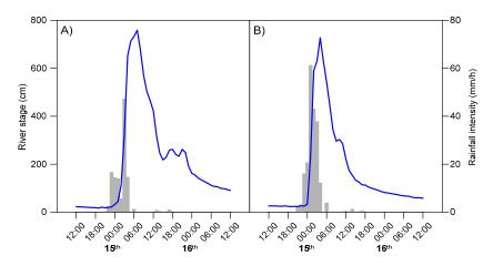
**Figure 8.** Storm hydrographs of the (**A**) Ponte Valentino (close to the ASI area) and (**B**) Pago Veiano stations. Figure 7 shows the station locations.
