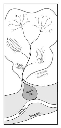
**Figure 14.** Schematic reconstruction of typical morphological structures of coalescent rills that induce debris flows identified in the study area: (**a**) Dendritic arrangement; (**b**) subparallel rill systems, parallel to the direction of the main creek; (**c**) subparallel rill systems, orthogonal to the main creek; (**d**) subparallel rill systems, directly flowing into a high-order gully (**e**).
