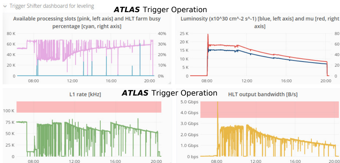
Figure 18. An example of a P-BEAST dashboard as used by the shifters during 2017 operation. The HLT farm availability (top left), the luminosity and the pile-up, 'mu' (top right), the total L1 accept rate (bottom left), and the total HLT output bandwidth (bottom right) are shown.
