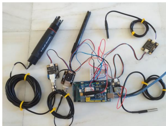
Fig. 1: The Arduino-based water sensor kit, that was used for the education activities.
