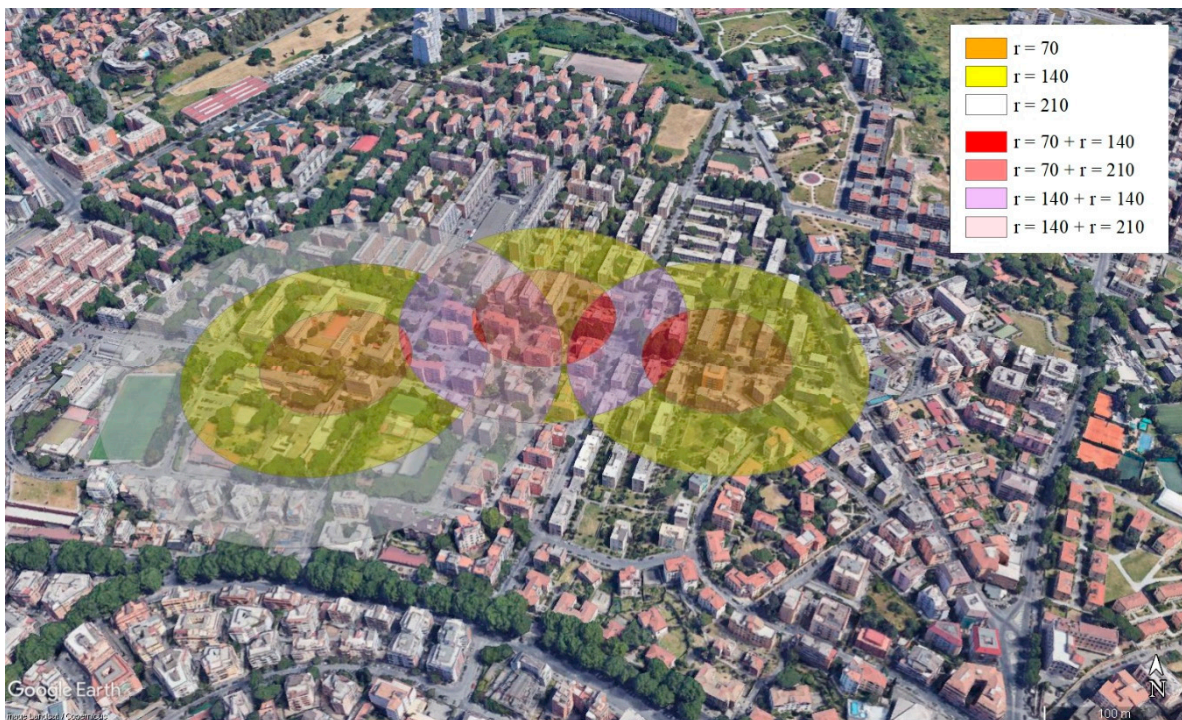
Figure 10. Prime three-dimensional model concerning the circular buffer zones defined by different radio base stations (the same as in Figure 8) in a GIS environment. Source: authors' elaboration.
