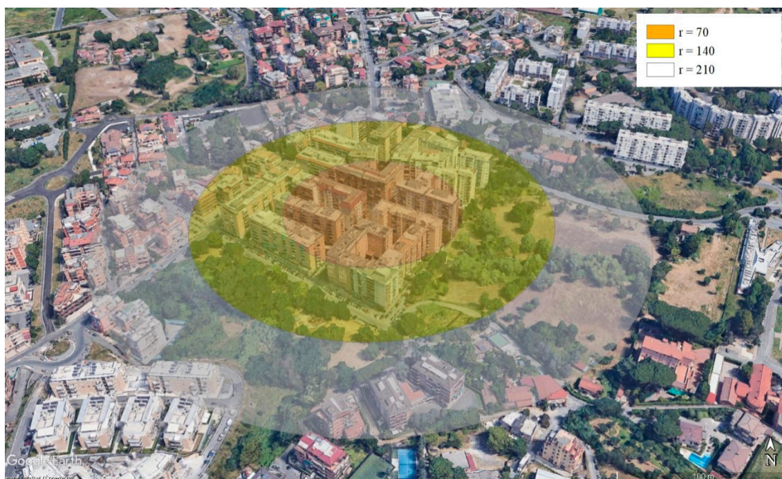
Figure 6. Prime three-dimensional model concerning the circular buffer zones defined by the imposing high antenna (the same as in Figure 4) in a GIS environment. Source: authors' elaboration.
