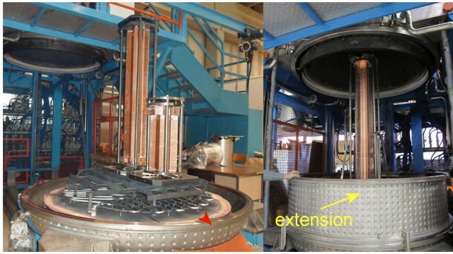
FIG. 7. Two half structures before brazing (left); full assembled structure in the INFN-LNL oven with the not-heated extension (right).
