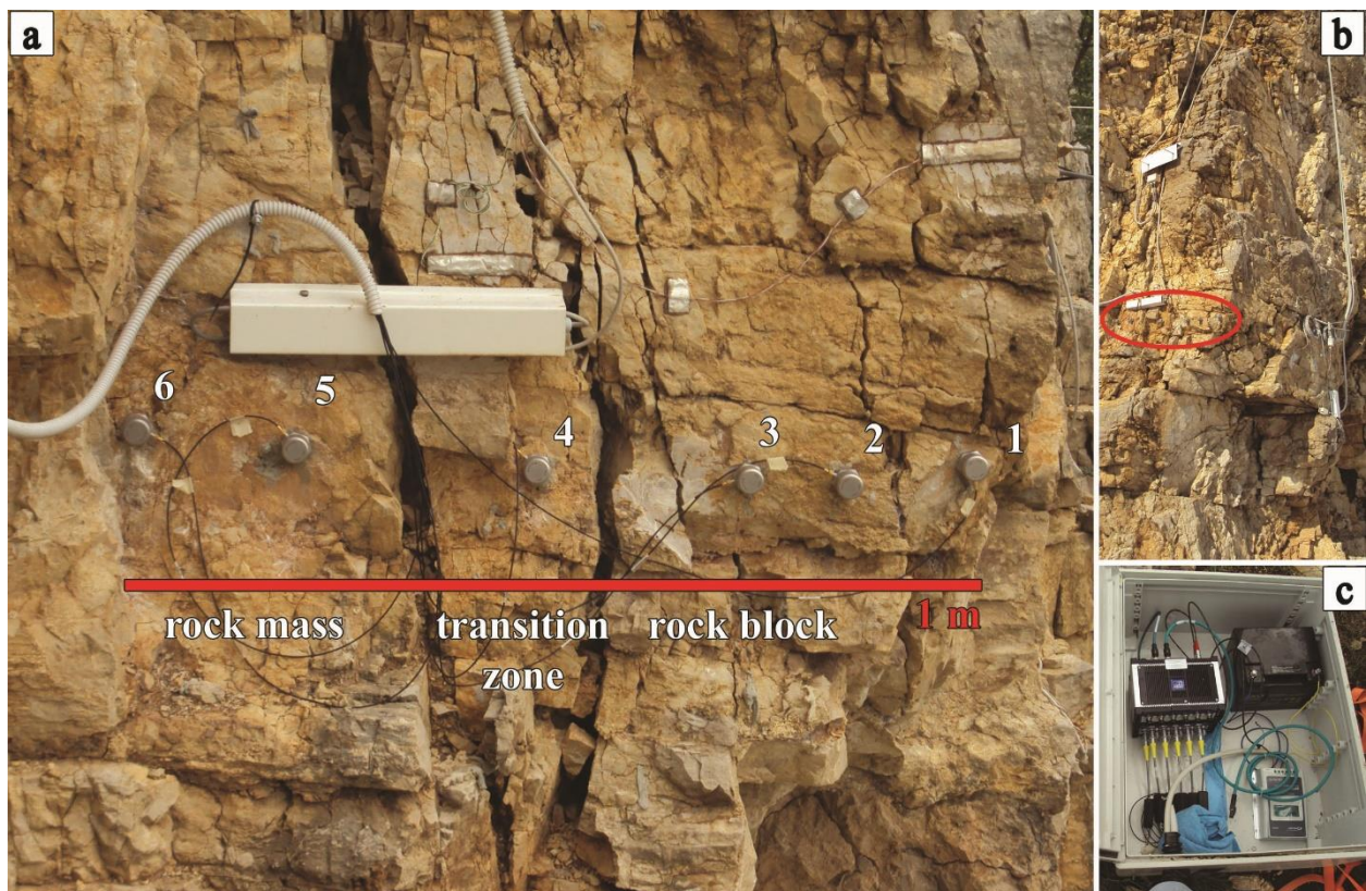
Figure 11: Positioning and ID of the accelerometers for the first microseismic monitoring campaign (Acuto 2018) (a). The location of the sensors on the rock block side is also shown in the circled area in b). The digital acquisition system and the backup battery were put into a watertight box placed on the top of the slope wall (c).
