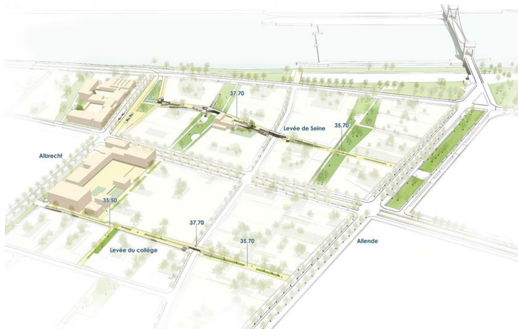
Figure 23. Vitry: a network of elevated paths connected by walkways allows the connection of urban services and entrances of residential buildings in the event of an extraordinary flood, while public spaces are designed to adjust to ordinary floods and violent rains. © Germe&Jam.
