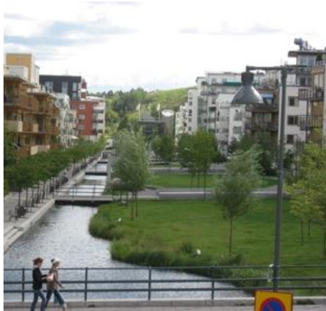
Figure 20. Hammarby: the new district recovers the riparian areas, purifies the waters of the lake with phyto-depuration systems and builds a network of canals and green corridors for rainwater that crosses private and public spaces of the neighborhood and connects both the woods and lake ecosystems.
