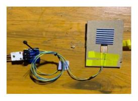
Figure 3: The Captec Radiant Flux sensor.
