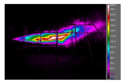
Figure 4: IR image of flame for test at 3 mm orifice and 325 bar (Temperature in K).
