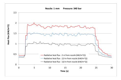
Figure 5: Heat Flux for 1 mm orifice at 340 bar.
