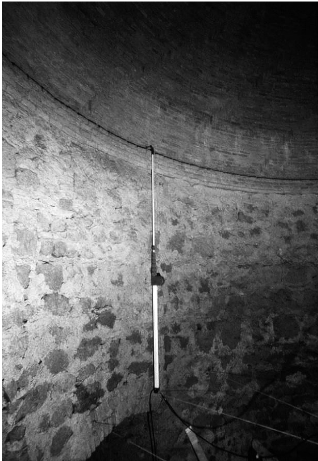
Fig. 30. Traditional survey, according to the Renaissance system used by Antonio da Sangallo il Giovane. Photo by C.B. 1985.
