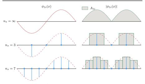
**Fig. 2** Representation of  $|\phi_{1i}(x_k)|$  for different values of the number  $n_s$  of sensors
