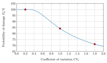
Fig. 6 Variation of the probability of damage  $P_d$  with the coefficient of variation  $CV_{\varepsilon}$ ; red dots are the values chosen for the application  $(CV_{\varepsilon} = \{0.2, 1.0, 1.8\})$
