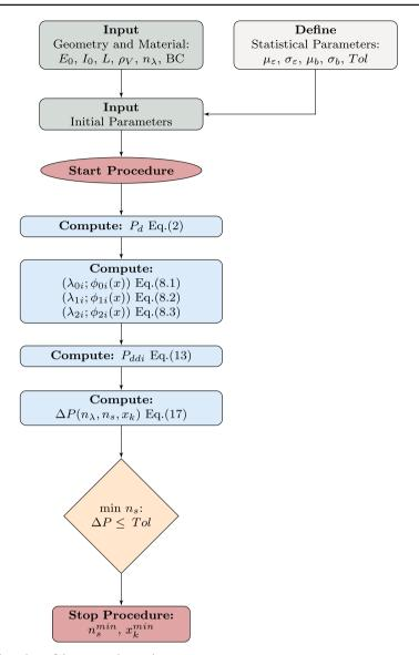
Fig. 3 Flow-chart of the proposed procedure
