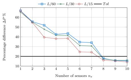
Fig. 7 Selection of the optimal number of sensors for the cases: four eigensolutions ( $n_{\lambda}=4$ ), coefficient of variation equal to 0.20 ( $CV_{\varepsilon}=0.20$ ) and three different spatial amplitudes  $\sigma_b=\{L/60,L/30,L/15\}$
