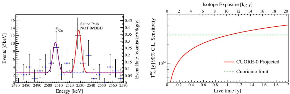
Fig. 3. Left:  $0\nu\beta\beta$  energy region of interest. The peak at 2506 keV is due to the sum of the two  $\gamma$ s from  $^{60}\text{Co}$ . The peak at 2528 keV is the salted  $0\nu\beta\beta$  peak (see text). Right: Projected sensitivity to the  $0\nu\beta\beta$  half-life.
