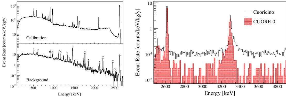
Fig. 2. Left: calibration and background spectra from threshold to 2.7 MeV. The peaks labeled in the background are due to  $\gamma$ s from (1)  $e^+e^-$  annihilation, (2)  $^{214}\text{Bi}$ , (3)  $^{40}\text{K}$ , (4)  $^{208}\text{Tl}$ , (5)  $^{60}\text{Co}$  and (6)  $^{228}\text{Ac}$ . Right:  $\alpha$  continuum background compared to Cuoricino. The peak at 3.2 MeV is due to  $^{190}\text{Pt}$  contamination in the crystals.
