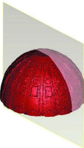
Fig. 24 2D study of the dome of St. Peter: radial profiles
