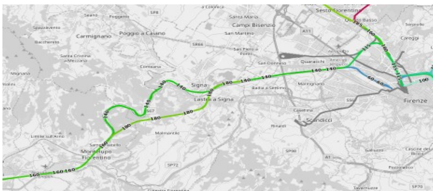
Fig. 3: Map of line with several curves of different radii suitable for the low-radius tests (TZ4) according to EN 14363.
