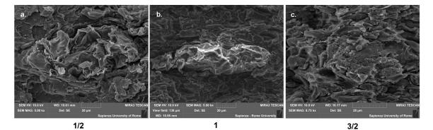
Figure 9. Leather particles embedded in the TPS matrix, 1/2 (a), 1 (b) 3/2 (c).
