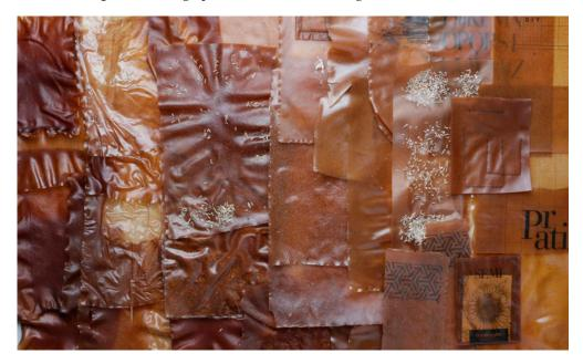
Figure 4. Coupling of the different films strips with lawn seeds prepared for application.
