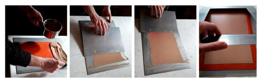
Figure 2. The different phases of the film casting.
