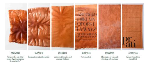
Figure 1. Experimental process leading to the development of the film.
