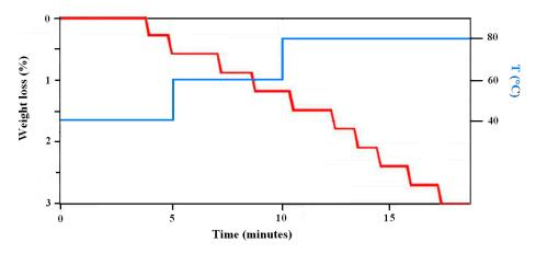
Figure 12. Weight loss of the material during heating up to 80 °C.
