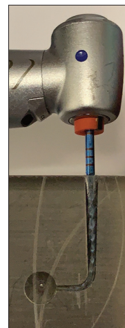
Figure 1: Device used with the instrument engaged in the artificial, stainless steel canal
