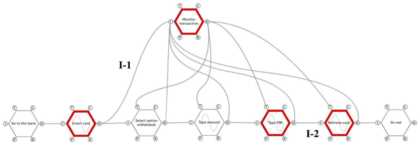
Fig. 2. FRAM instantiation of the cash withdrawal case study. Notes: (i) functions in red are those selected for analysis; (ii) waves inside the hexagons indicate variability in the function's output. (For interpretation of the references to colour in this figure legend, the reader is referred to the Web version of this article.)
