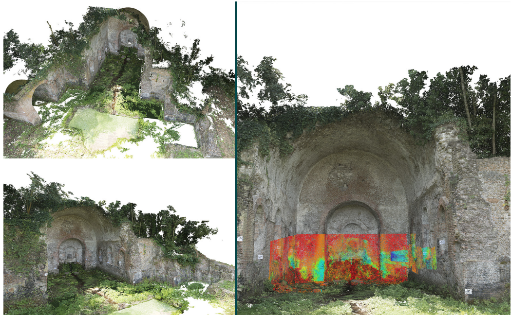
Fig. 3. On the right, the point cloud generated by SfM processes, on the left, integration with point cloud generated from thermographic images [Griffo, Cimadomo, Menconero 2019].
