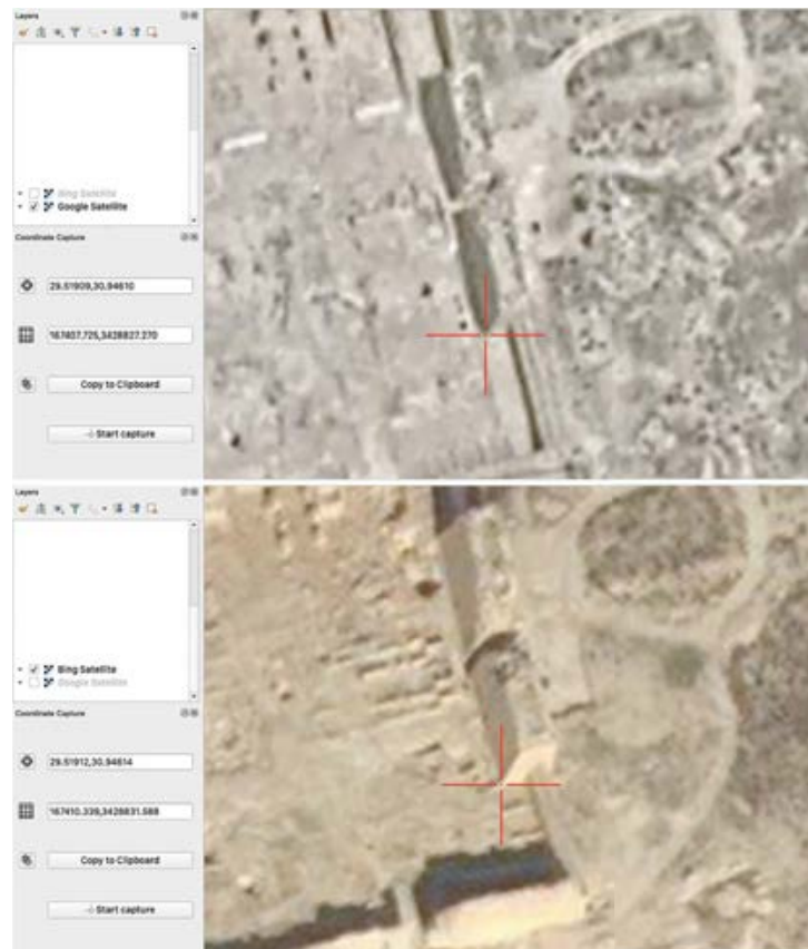
Fig. 3. Comparison of the coordinates of the same, clearly recognisable ground control point: the base of the southern pylon of the temenos of Taposiris Magna (paths.place:338). The upper image is imported from Bing and the lower one from Google satellite images. Coordinates are expressed in the same projection system, WGS 84/ UTM zone 36N (EPSG: 32636). The linear difference can be calculated to more than 5 meters.
