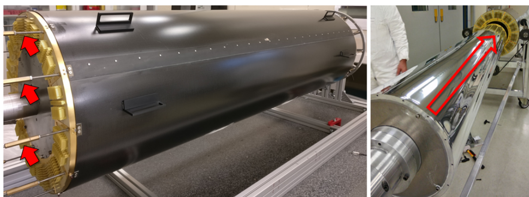
Figure 3. Left: the CF support structure with some turnbuckles highlighted. Right: insertion phase of the 20 \mu\text{m} Al Mylar foil.
